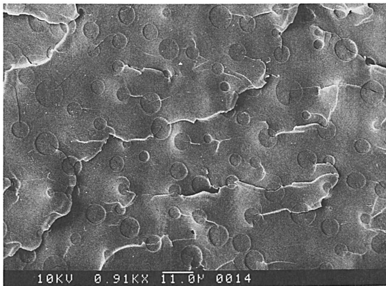
Figure 7. SEM of the 828-PIP-1300×21 formulation cured at 120 °C.
